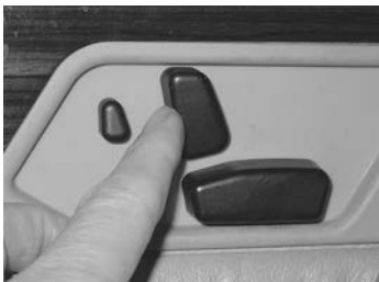
FIGURE 1.7. Good Mapping: Automobile Seat Adjustment Control. This is an excellent example of natural mapping. The control is in the shape of the seat itself: the mapping is straightforward. To move the front edge of the seat higher, lift up on the front part of the button. To make the seat back recline, move the button back. The same principle could be applied to much more common objects. This particular control is from Mercedes-Benz, but this form of mapping is now used by many automobile companies. (Photograph by the author.)
